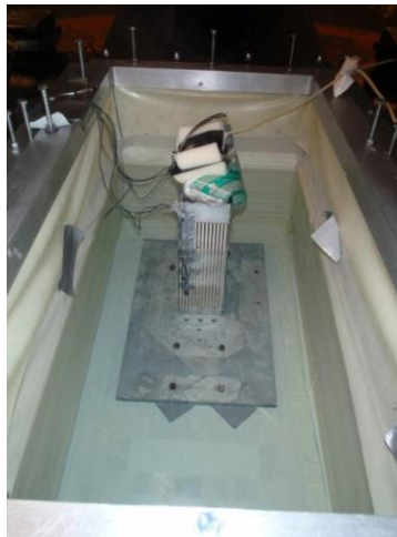
Figure 4.2. Centrifuge water tests performed at RPI to calibrate tactile pressure sensors (Olson et al. 2011).
