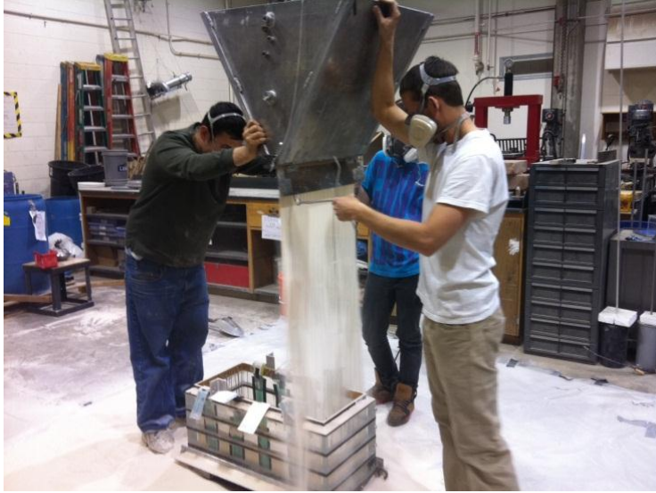
Figure 5.5. Dry pluviation of Nevada sand over tactile pressure sensors in the centrifuge container.
