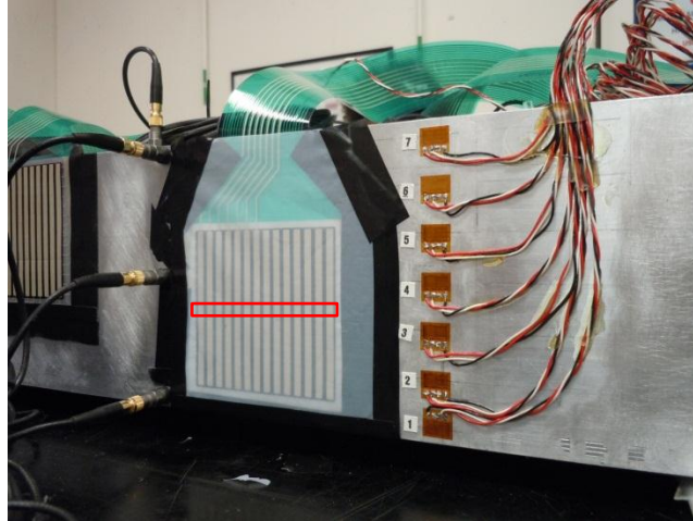
Figure 5.9. Centrifuge testing configuration of tactile pressure sensor on tunnel wall. Sensel readings in each row were averaged.
