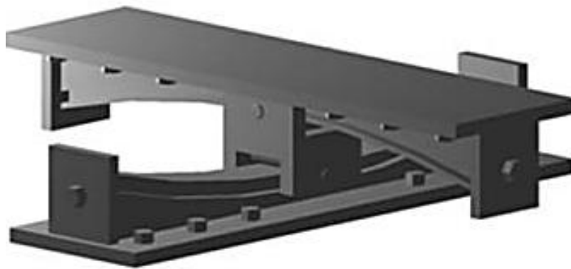
Figure 19: UR-FPS Isolator (Fardis, 2010)
