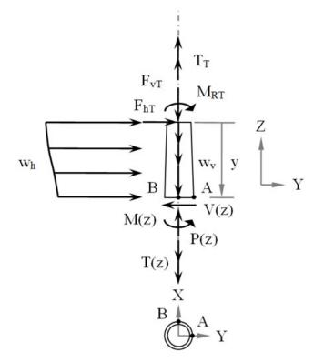
Figure 3-5. Location of critical points A and B
