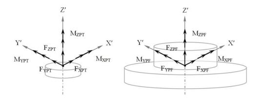
Figure 3-1. 3-dimensional force components at tower top and foundation
