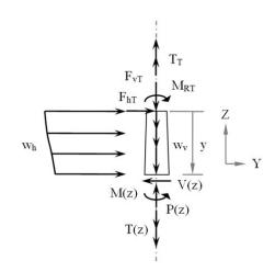
Figure 3-4. Free body diagram of tower section
