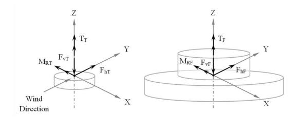
Figure 3-2. 2-dimensional resultant forces at tower top and foundation
