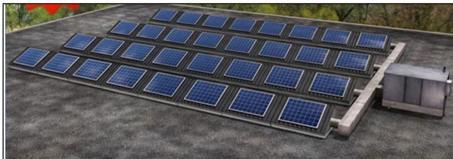
**Figure 1.** This is a rendering of the SolarDuct modular system. The PV modules are mounted on top of the SolarWall and air is drawn in behind the PV and into the building air handler. (SolarWall, 2012)
