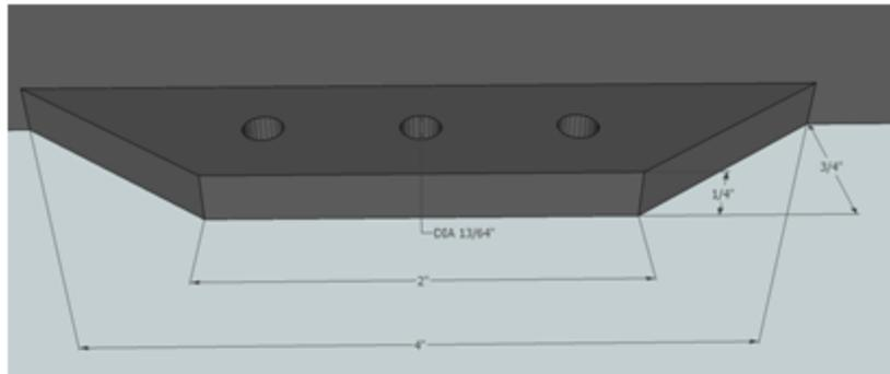
All mounting flanges on headers and side rails are the same. The center screw hole is centered, and the flanking screw holes are  $\frac{3}{4}$ " on center from center hole. Diameter is about 0.2", to accommodate a #10 wood screw at a 72 degree angle.
