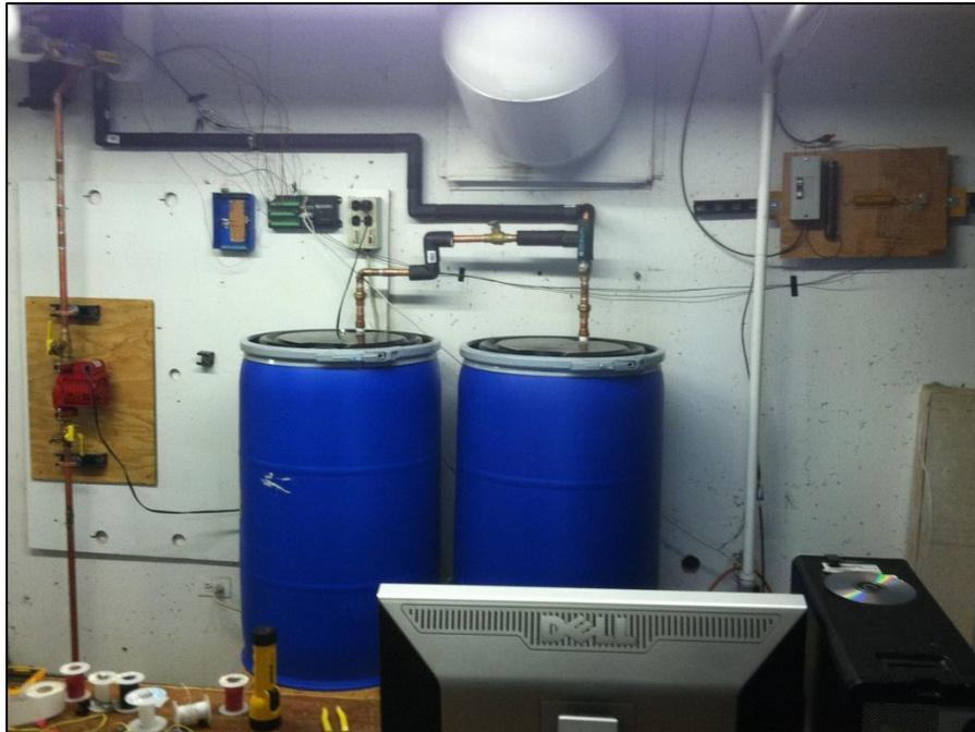
Figure 30. This is a photo of the experiment from inside of the Larson Lab. In the upper right hand corner is the electrical terminations and PV load dumping station. Centered in the photo are the two 55-gallon tanks, and the datalogger and thermistor enclosure. The 1/6 HP circulator pump is seen in the left hand side of the photo.
