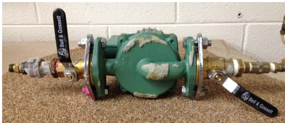
Figure 3.8: Taco Model 009-F5 high velocity centrifugal pump (cartridge circulator) used in-series with Julabo heat pump to increase flow through system
