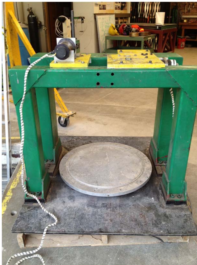
Figure 3.10: Loading frame for the 400 g-ton geotechnical centrifuge
