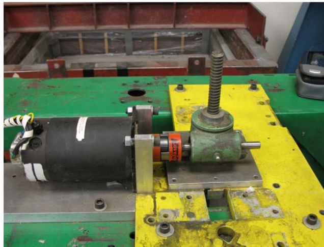
Figure 3.11: Brushed DC motor used to apply building load to model foundation
