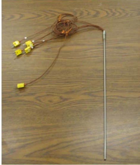
Figure 3.15: Photograph of a thermocouple profile probe
