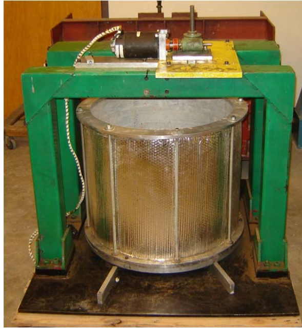
Figure 3.12 Soil container within the load frame
