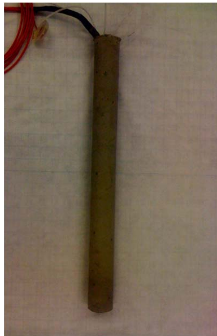
Figure 3.2: Photograph of a scale-model energy foundation; heat exchanger tubes and cables from embedded instrumentation are seen at top
