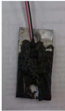
Figure 3.6: Strain gage attached to steel tab and covered with epoxy
