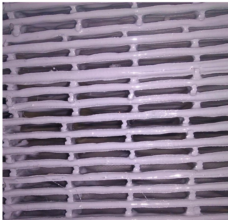
Figure 24. Front (inlet) side of HMX, close-up; Note the wide variance in open channel heights and non-uniform inlet shape due to epoxy sealant.
