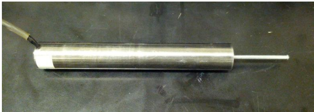
Figure 4.8: LVDT used to measure the axial deformations
