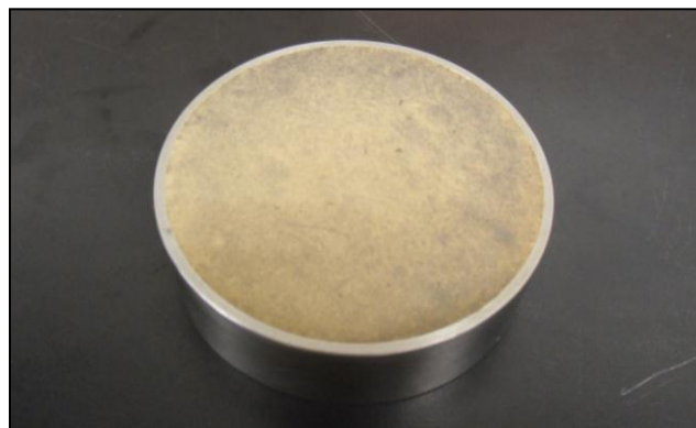
Figure 5.4: Compacted Bonny silt specimen
