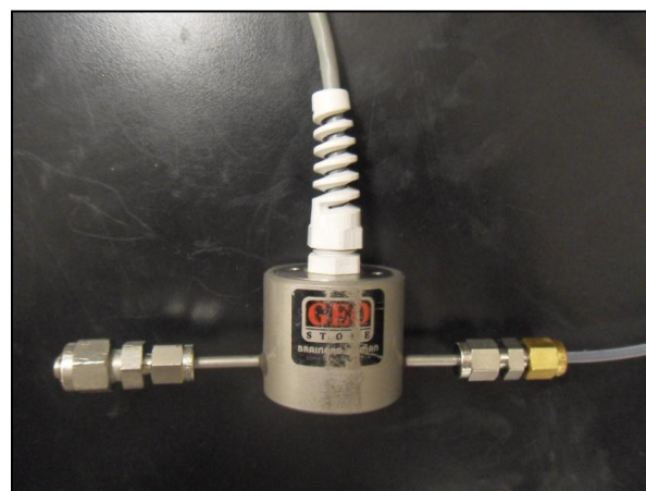
Figure 4.11: Pore water pressure transducer
