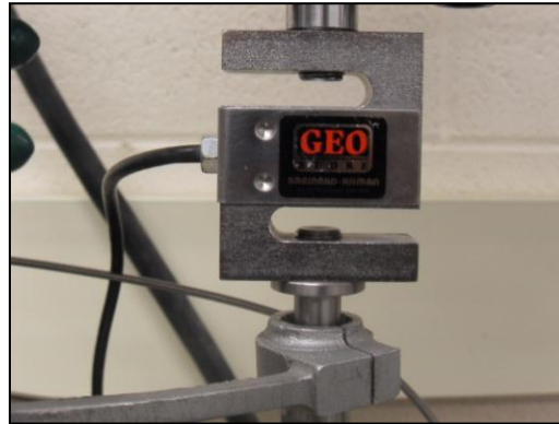
Figure 4.7: Load cell used to measure the axial load applied to the specimen
