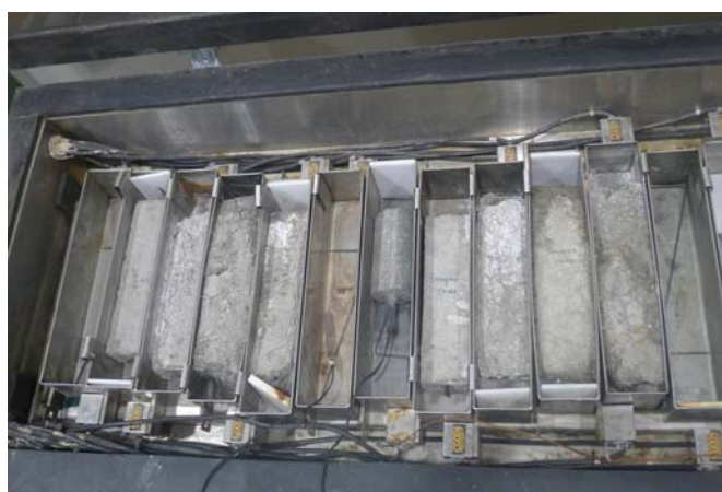
Figure 3.11 Logan Rapid Freeze-Thaw Chest
