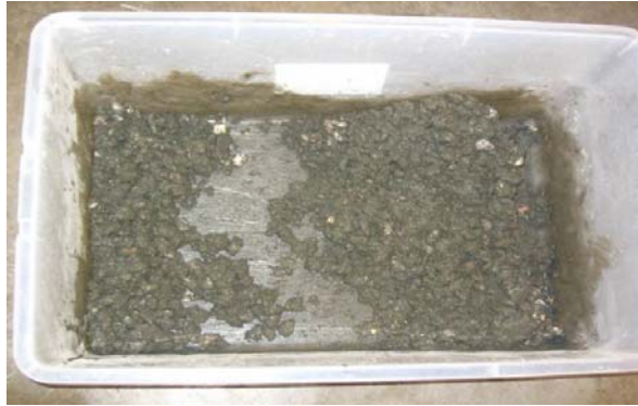
Figure 2.4 Surface treatments with cement slurry plus silica fume in Group 4
