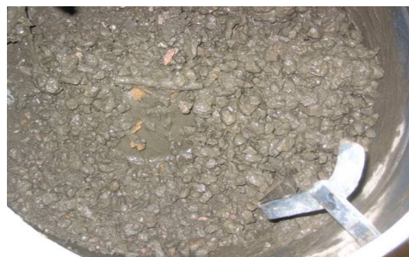
Figure 2.15 Mixing approach 3: two-stage mixing approach (TSMA)
