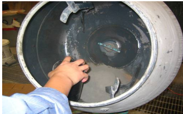
Figure 2.13 Mixing approach 1: mortar mixing approach (MMA)
