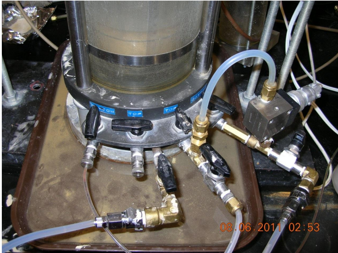
Figure 2.2.2 – shows a typical SICT setup; Top photo – the slurry is poured into a plastic cylinder; Bottom photo –a gradient created across the specimen using a flow pump. The valves at the bottom of the triaxial cell control water flow into and out of the sample, also note there is a pressure transducer at the bottom
