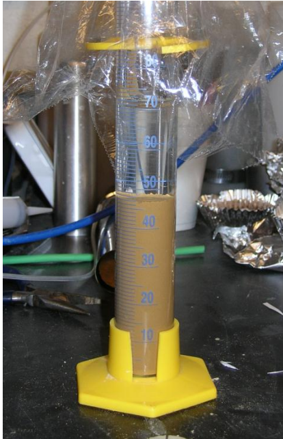
Figure 2.2.1 – a slurry sample being allowed to consolidate under its own weight, note some consolidation has occurred as evidenced by the water on top of the sample
