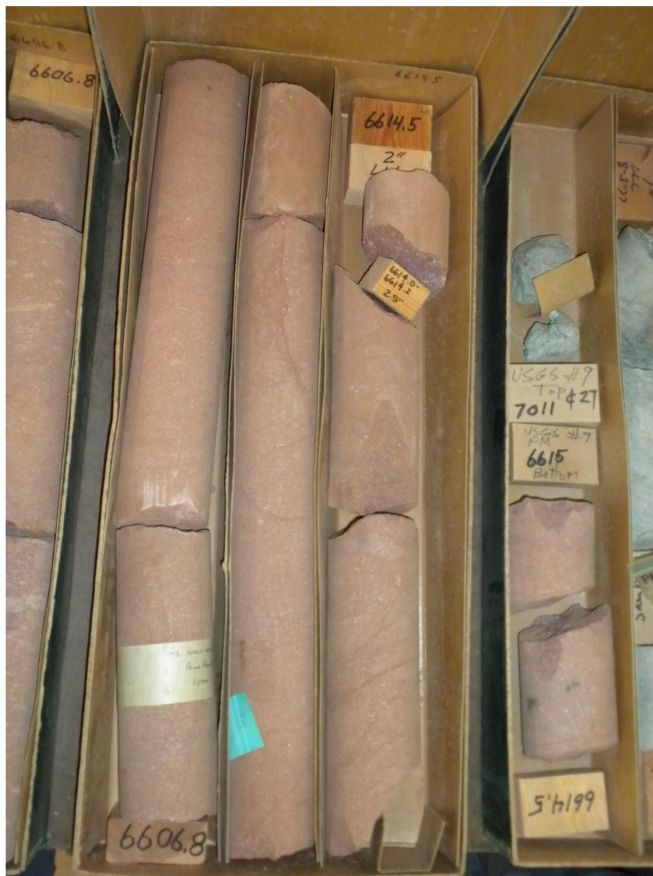
Figure 4-2. Box of drill core from the USGS Mercury Core Library showing a sample of interior intact core at 6614'
