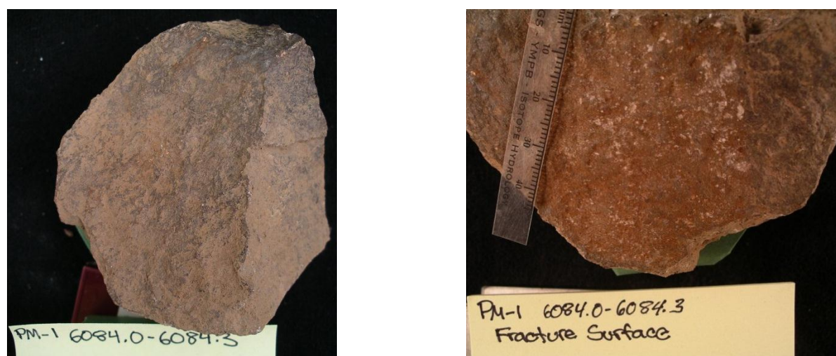
Figure 4-3. Illustration of discrete fracture before and after scrapping for PM-1:6084'
