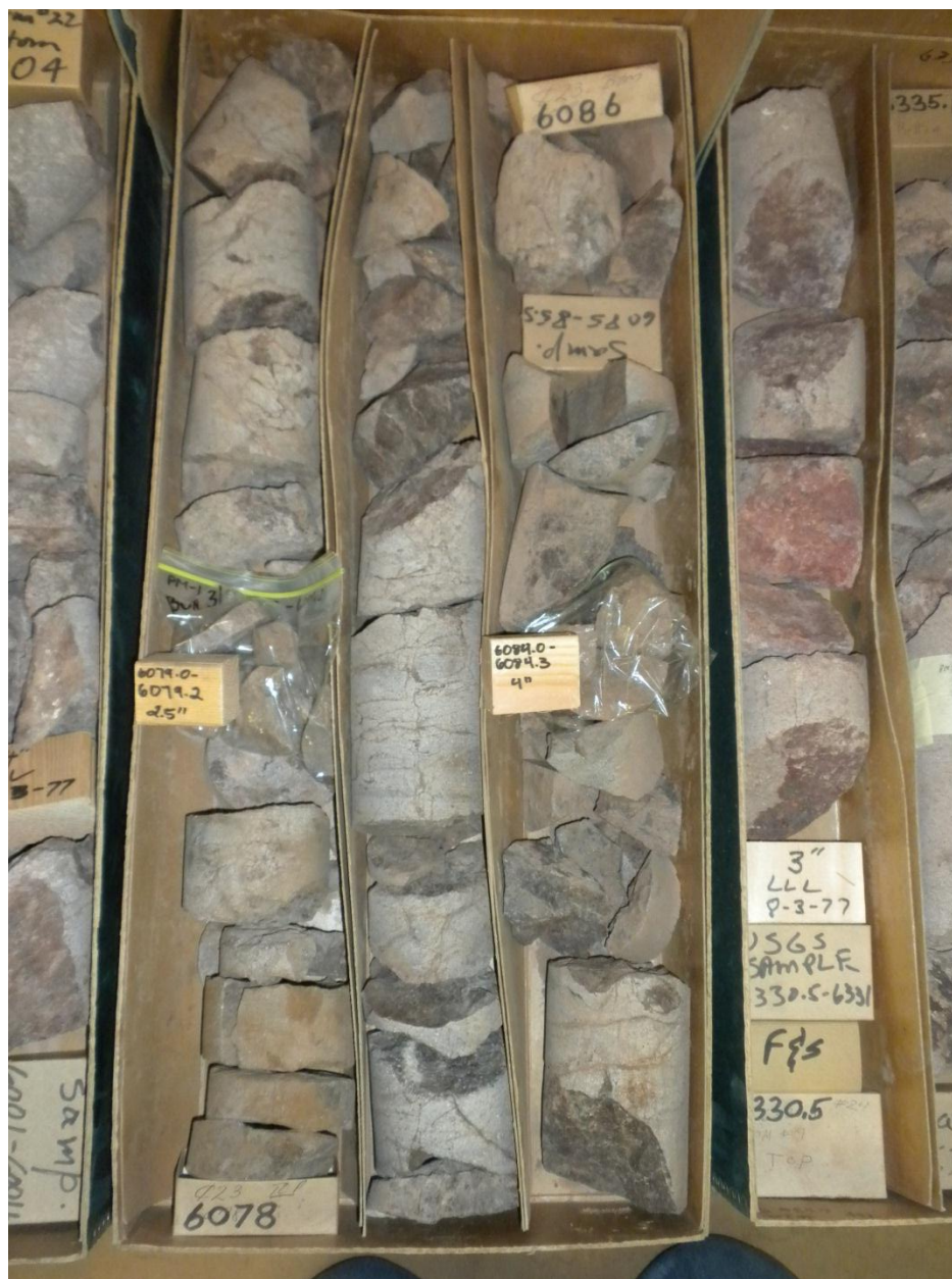
Figure 4-1. Box of drill core from borehole PM-1 at the USGS Mercury Core Library showing samples of a discrete fracture at 6084' and brecciated/rubblized core at 6079'
