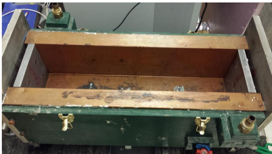
Figure 3 Free shrinkage frame empty
