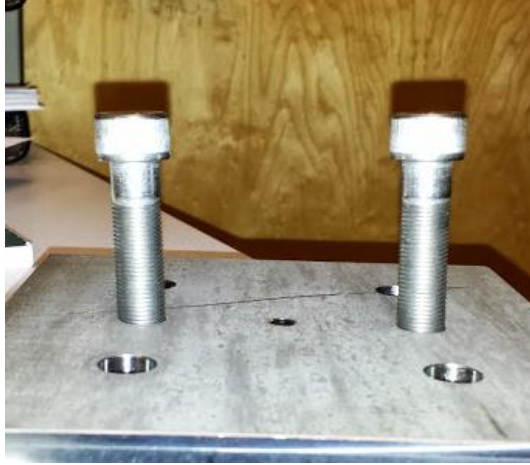
Figure A.3 Movable 6 inch x 6 inch x \frac{3}{4} inch thick stainless steel movable plate with bolts that drive the plate in and out for free shrinkage frame
