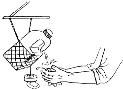
Figure 2.1: Tippy tap handwashing station (reproduced from CDC, 2013). Figure is from government website and public domain.
