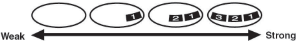
Figure 5. A three-segment display indicating four levels of signal quality.
