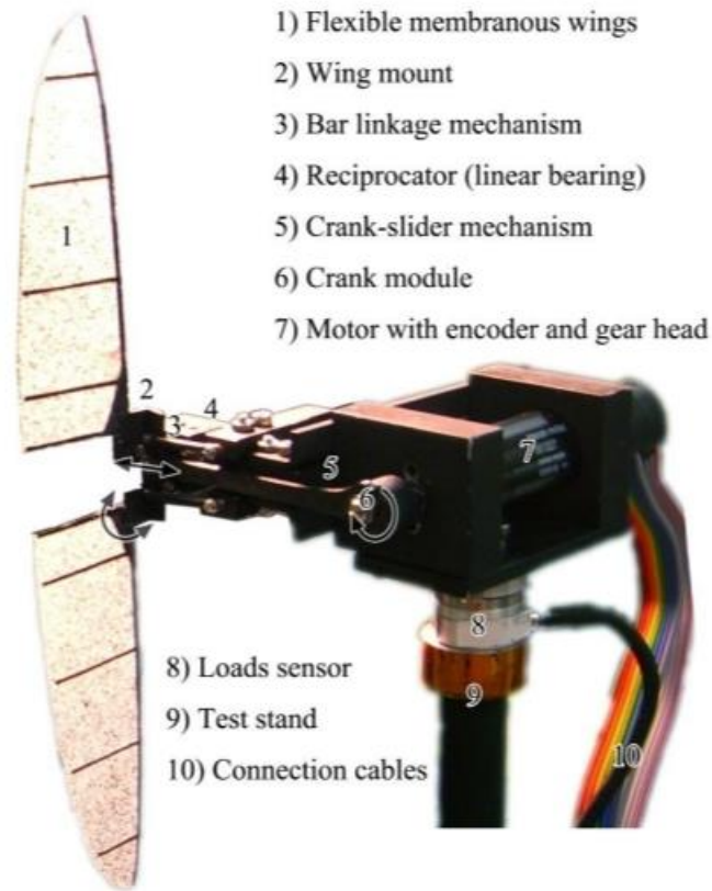
Figure 3.16: Flapping wing mechanism from Ref. [164]
