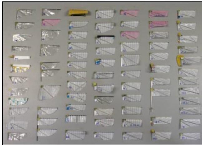
Figure 1.46: Sample set of test wings from the Nano Hummingbird program [51]
