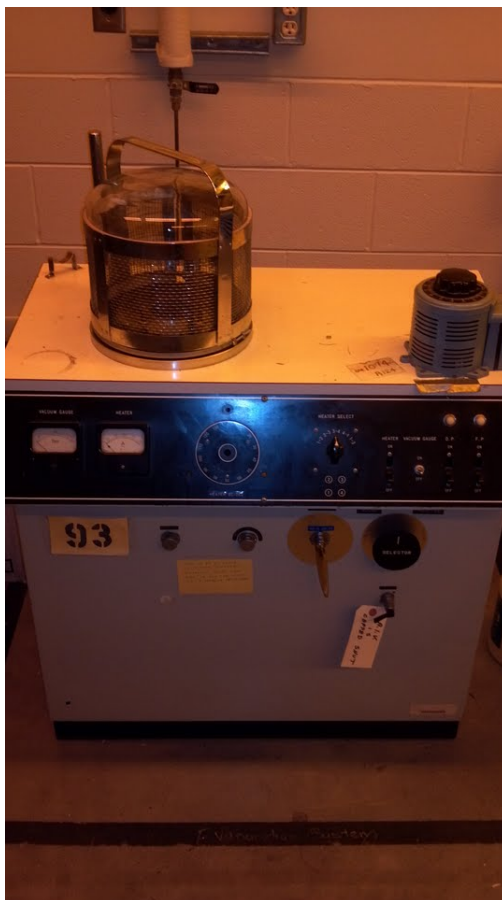
Figure 3.8: Hitachi HUS-4 Evaporator at Western Michigan University
