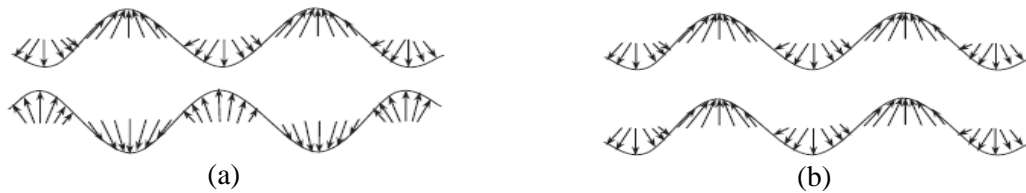
Fig. 2-1: Illustrations of the particle motions of (a) symmetric and (b) antisymmetric modes in the cross section of a thin plate [37]
