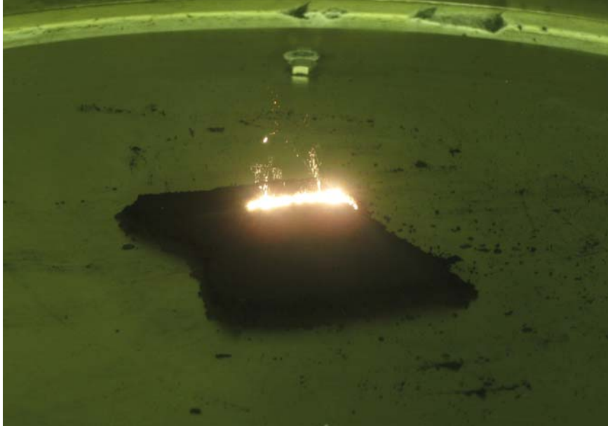
Figure 2.14 Visible radiation emitted during irradiation of carbon black by the CO 2 laser.
