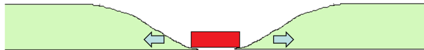
Figure 4-10. The shape of the tube as the first finger compresses the tube
