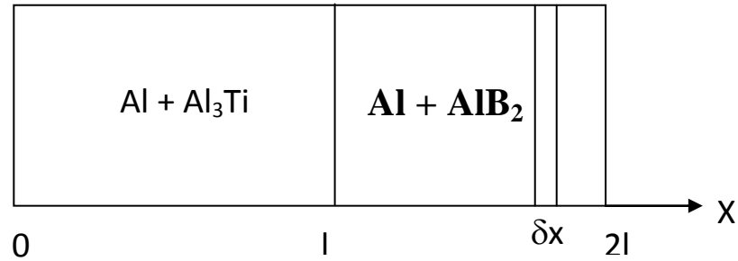
Figure 5.6: A schematic of the coordinate system used for precipitate modeling 82
