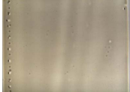
45 psi: thinning/holes, few bubbles
