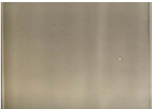
50 psi: nearly no defects
