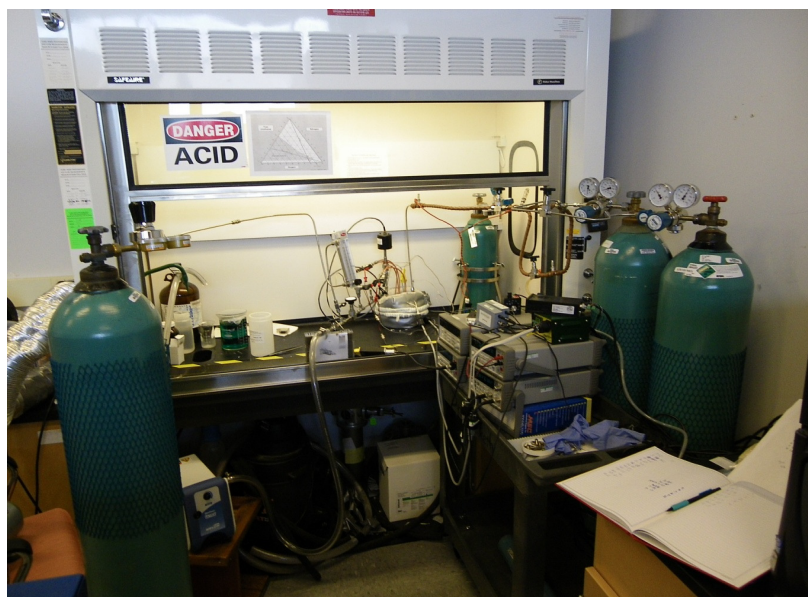
Figure 2.4. Gas cylinders connection to the QCM setup.
