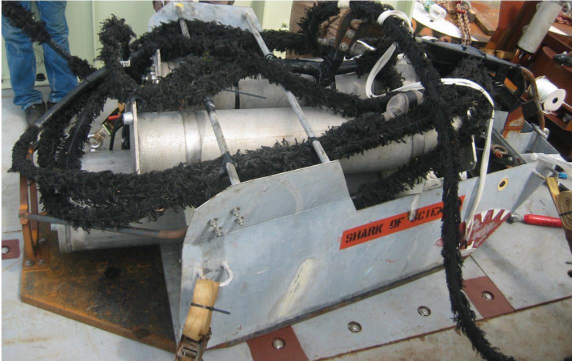
Figure 2.14 Shark electronics battery sled (Newhall et al. , 2007)
