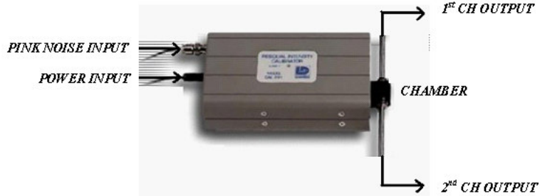
Figure 39: Larson Davis residual intensity calibrator
