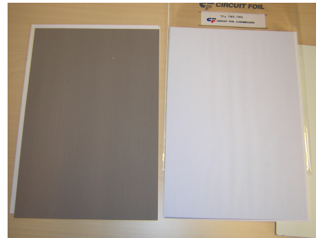
Figure 14: TWS 70 \mu\text{m} copper foil.
