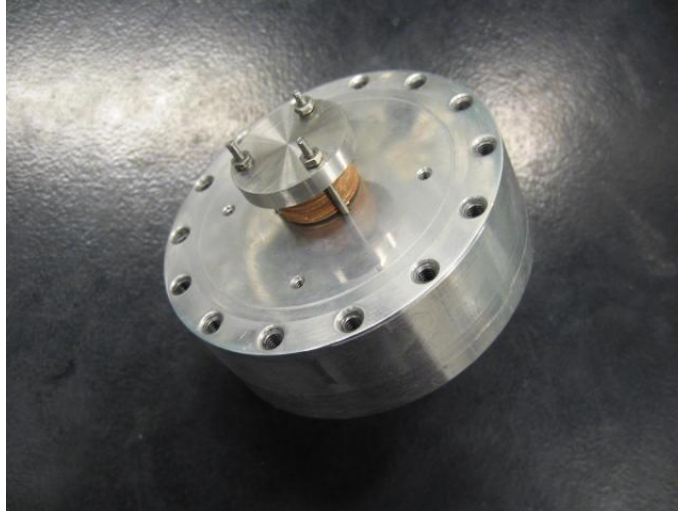
Figure 3.6 Photograph of #325 phosphor bronze radial flow sample mounted in test apparatus
