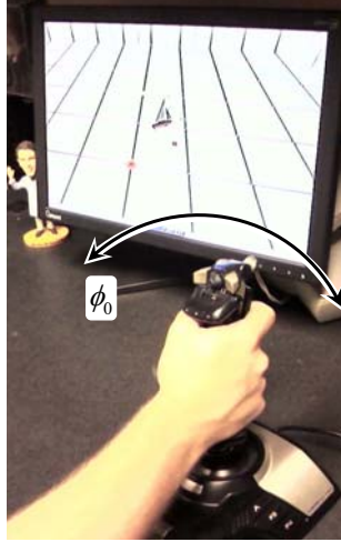
Figure 5.5: The operator video display and joystick
