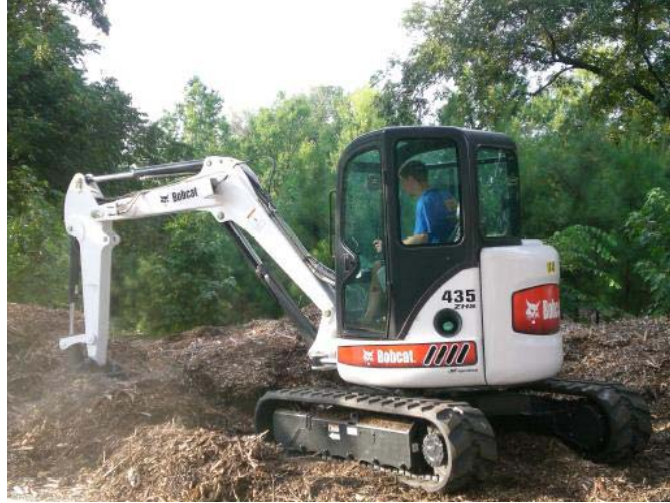
Figure 8.1: The Bobcat 435 compact excavator research testbed ( photo courtesy of Mark Elton )
