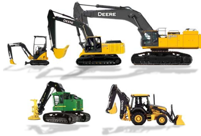
Figure 2.2: A group of machines kinematically similar to excavators. Clockwise from top left: compact excavator, construction excavator, production excavator, tractor-loader backhoe, log feller buncher. Shown in approximately equal scale. ( Images courtesy Deere & Co. )
