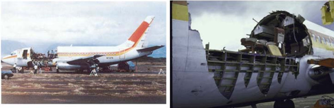
Figure 1-2 Complete structural failure of a 737 in Hawaii in 1988 (picture from internet)
