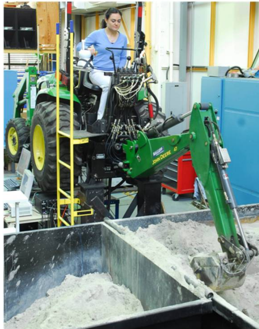
Figure 6: Haptically Enhanced Robotic Excavator (HEnRE) Testbed with SensAble Omni
