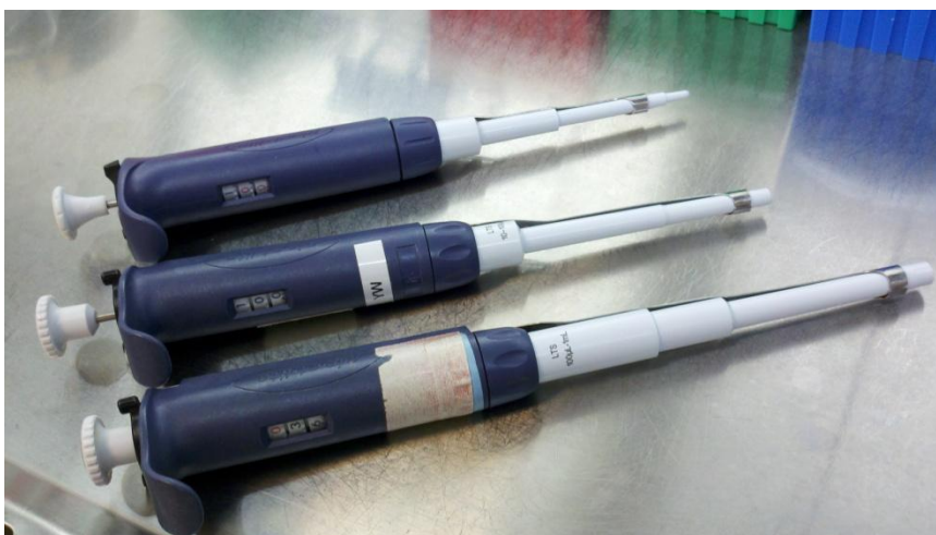
Figure 1 - Three different sized pipettes. The volume adjustment can be seen protruding from the top.
