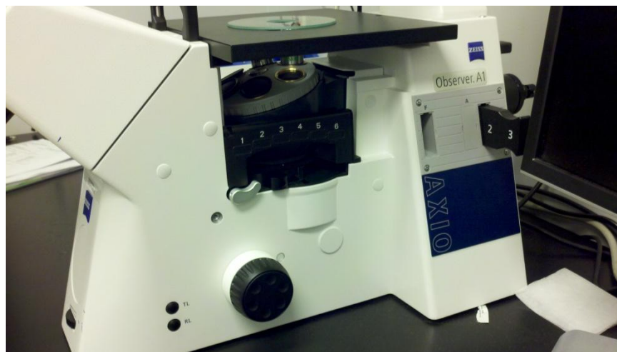
Figure 5 - Controls of fluorescence microscope, including TL/RL buttons, focus, and brightness adjustment on the front.
