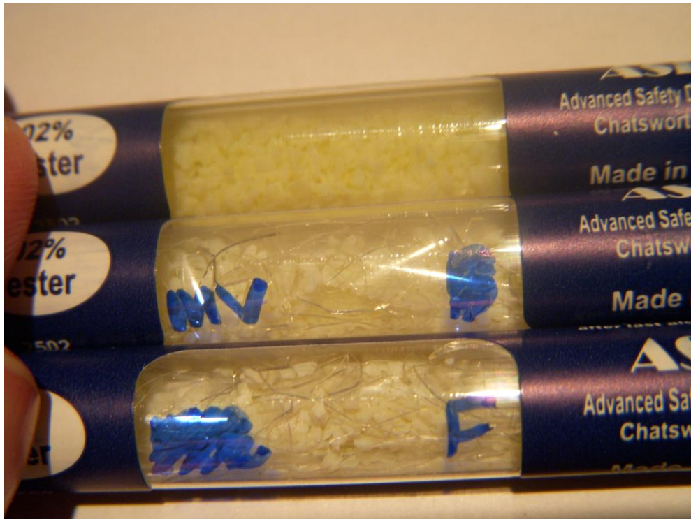
Figure 16. Measured volume results from the blood alcohol experiment. The tester on top is unused. The middle tester is the measured volume tester (MV), and the tester on the bottom (F) is a tester that was triggered when it was attached to the filter tube. The crystals in the control tester are very yellow, and the crystals in the MV and F testers are white.
