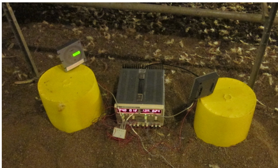
Figure 3.4. Image of the static flux buckets with small internal mixing fan used to measure CO 2 flux from the litter surface. CO 2 probe was on the top of the bucket and measuring approximately 6 cm from the top of the bucket.
