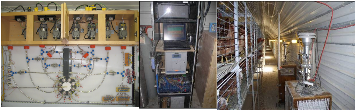
Figure 2.4. Gaseous and particulate matter (PM) concentration monitoring system (L- R: positive-pressure gas sampling system or P-P GSS, gas analyzers, and Tapered Element Oscillation Microbalance or TEOM PM monitors).
