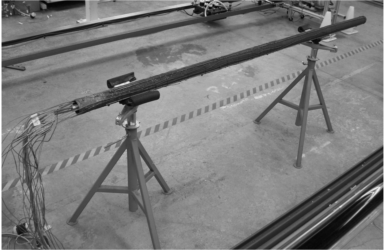
Figure 4.6 Heaters inside copper pipe
