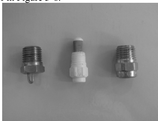
Figure 5-5. Spray nozzles used in this study, left to right: PJ20, 1/8SF-CE, 1/4M-8
