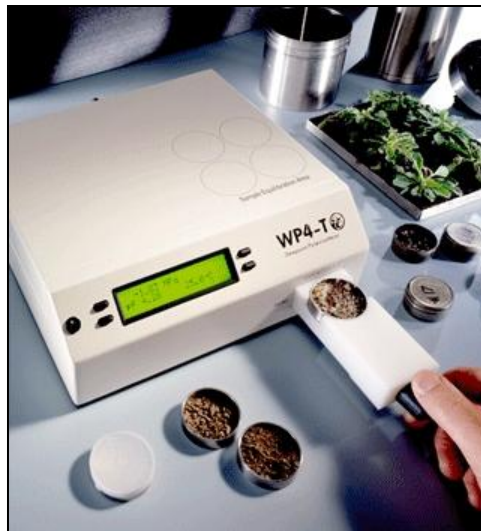
Figure 4.8. The chilled-mirror dew point device model WP4-T.
