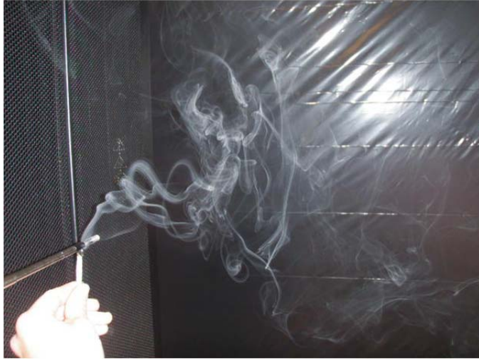
Figure 5–74: Flow visualization of airflow behind rack with top server simulators removed
