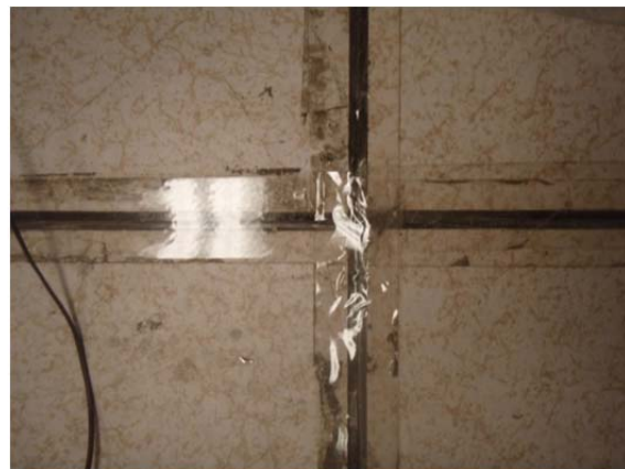
Figure 3–13: Sealing the test chamber ceiling and floor
