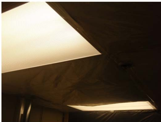
Figure 3–13: Sealing the test chamber ceiling and floor
