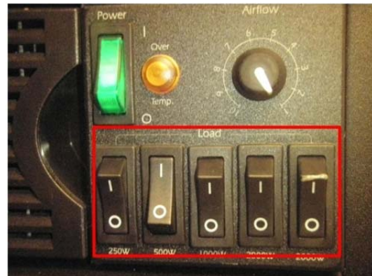
Figure 3–21: Heating Element Control Switches
