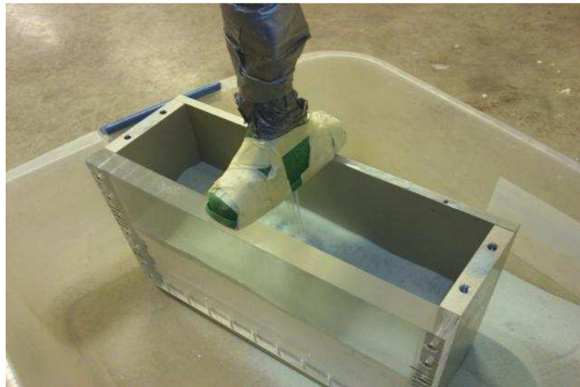
Figure 5.2 Preparing the sand layer by air pluviation.
