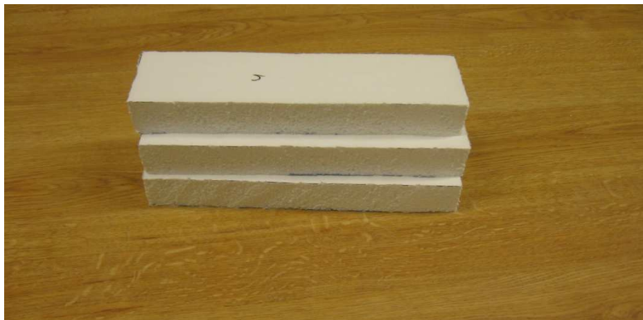
Figure 4.4 Styrofoam sheets (thick) used to represent the soft layers.
