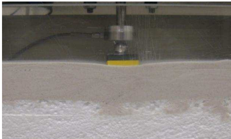
Figure 3.8 Picture of loads being applied to the footing.
