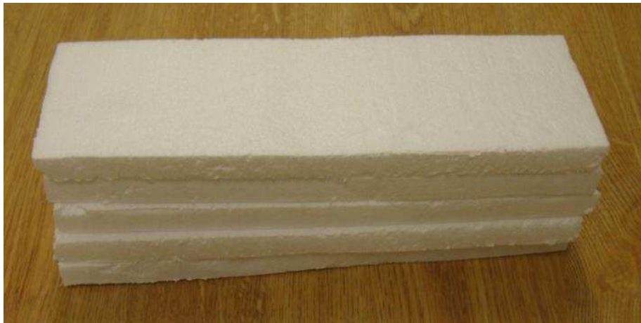
Figure 4.3 Styrofoam sheets (thin) used to represent the soft layers.
