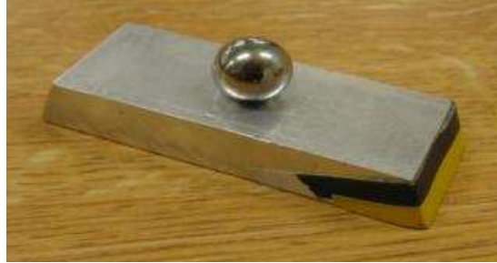
Figure 3.4 Footing with a yellow and black marker for digital image analysis.
