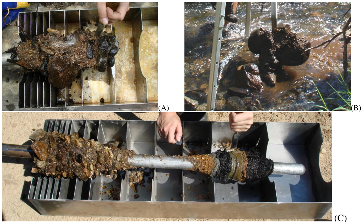
Figure 2.18. Sediment cores collected at (A) 23 m, (B) 42 m, and (C) 77 m. The core at 42 m is pictured as it was being hoisted from the sediment. We were able to immobilize large rocks as well as fine sediments using the freeze core method. The sediment is missing from about 35 – 55 cm from the core collected at 77 m, possibly due to uneven freezing along the pipe. Partitions on the tray were 2 cm wide for the first 10 cm, then 5 cm wide from 10 cm-20 cm, then 10 cm wide for the 30-60 cm, and 20 cm wide for the remaining 40 cm.
