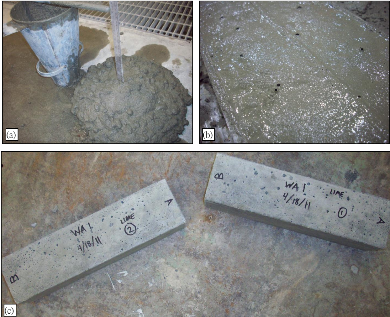
Figure 3-18. (a.) Increased concrete slump using surfactant. (b.) Bubbles present in fresh concrete (c.) Bubbles present in hardened specimens.
