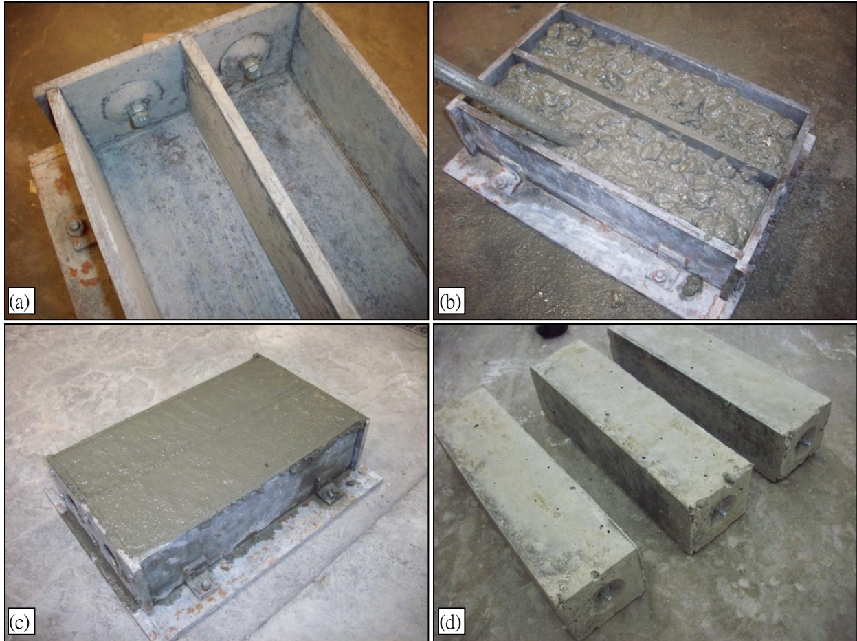
Figure 3-5(a). Molds with gauge studs. (b). Tamping to consolidate specimens. (c). Smooth top surface formed by trowel. (d). Demolded specimens.
