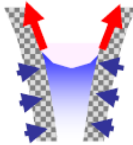
Figure 1-3. Schematic illustration of capillary forces within material pores (Asamoto, Ishida, & Maekawa, 2008).
