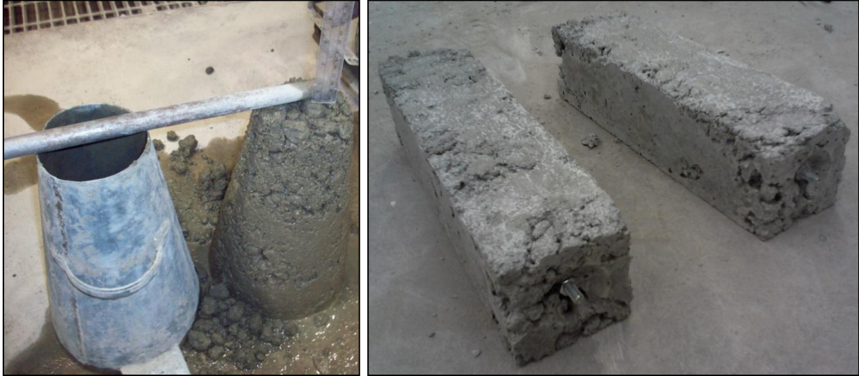
Figure 3-17. Voids present in 100% silica cement treated RCA due to reduced workability.
