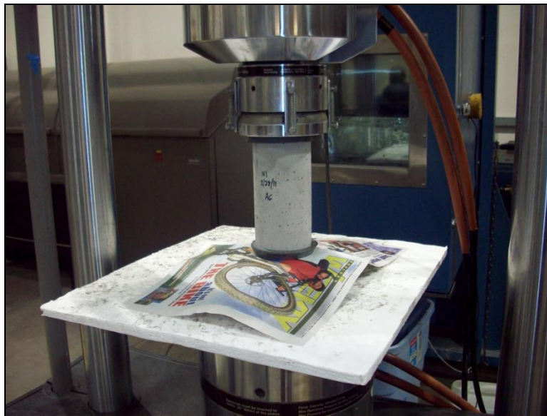
Figure 3-3. Concrete cylinder compression test.
