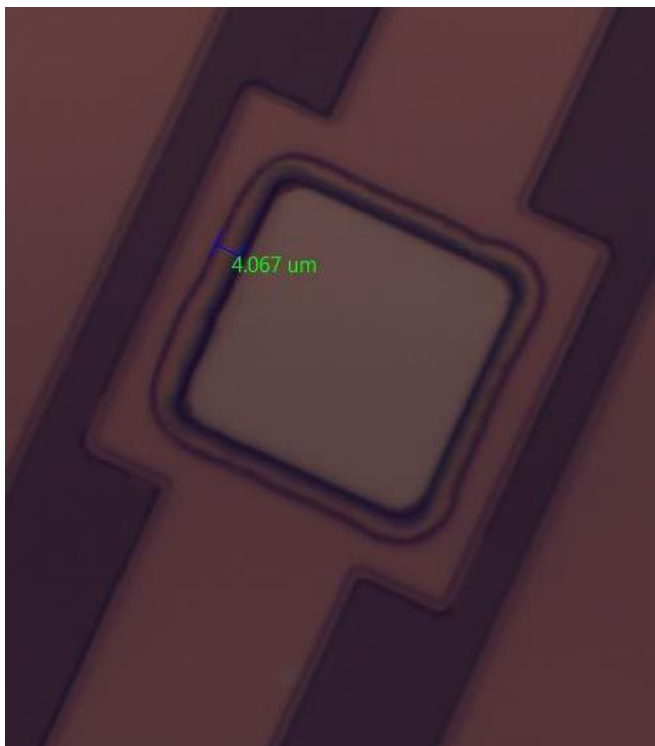
Figure 37. Top-view photo showing undercut observed after 5 minutes of BOE wet etch.
