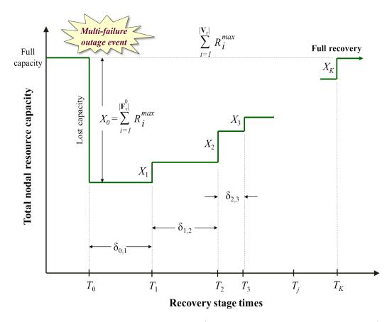
Figure 3.3: Progressive recovery stages (aggregate datacenter node resource)
