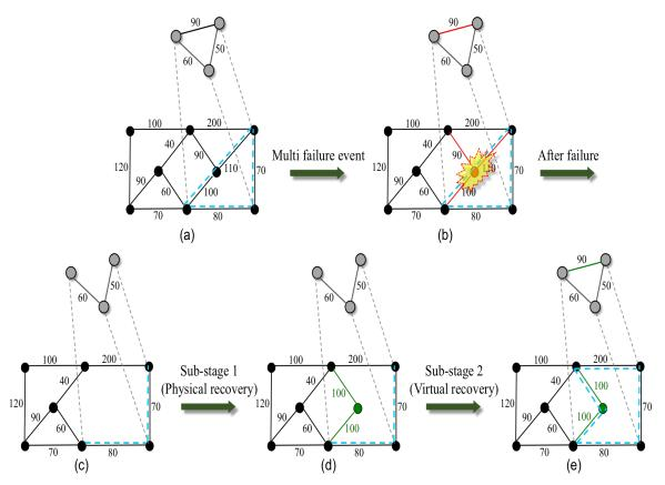
Figure 3.4: An example of dual-stage progressive recovery scheme
