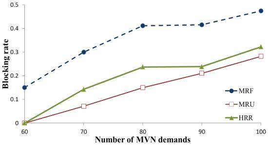
Figure 5.5: Blocking rate for 24-node network
