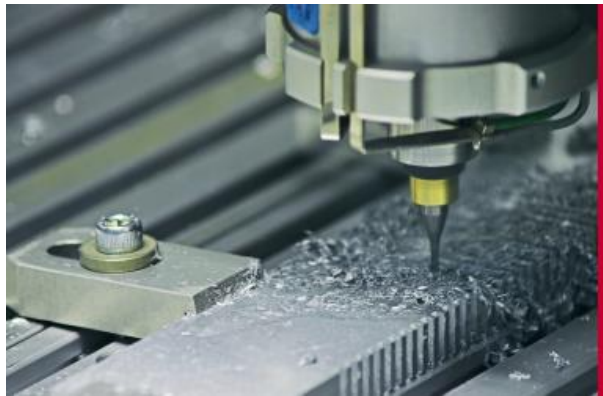
Figure 2.3 Computer controlled machining (top-down process)[69].
