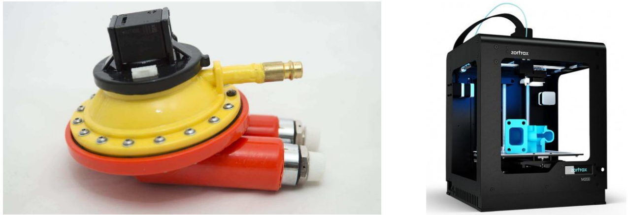
Figure 7.5 Artificial heart on the left and the Zortrax M200 3-D printer used to create it[87].
