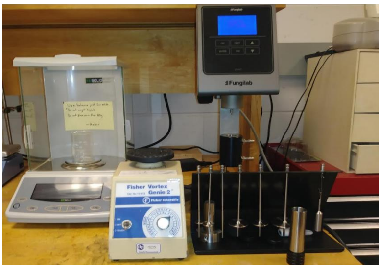
Figure 8.13 Left to right: Microscale, vortex mixer and viscometer with attachments.
