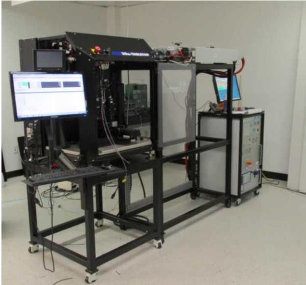
Figure B.1: nScript Tabletop 3Dn printer.
