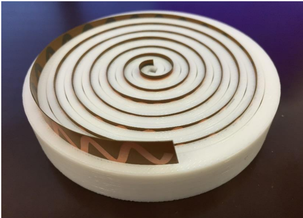
Figure 3.4. Additive manufactured Polycarbonate dielectric with PSA element partially installed.
