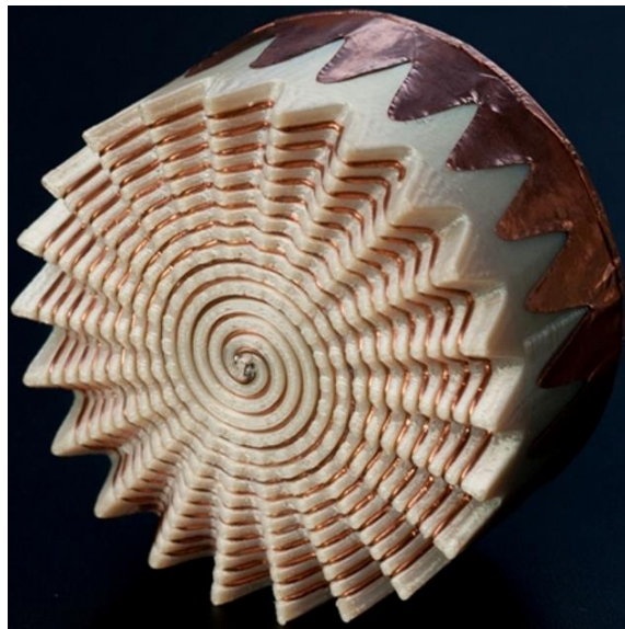
Figure 3.2. Fabricated model of sinuous cavity backed PSA antenna utilizing an exponential growth factor of 3.
