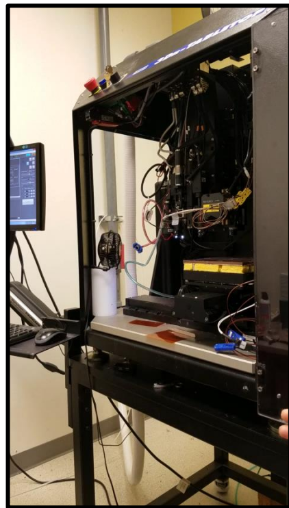
Figure 1.1 - Tabletop Series nScript Material printer used to conduct the experiments presented.
