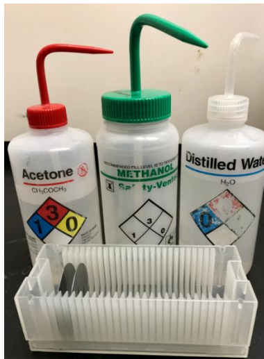
Figure 4.2: Chemicals for Acetone-Methanol cleaning, in fumehood, Surface Science Laboratory, University of South Florida
