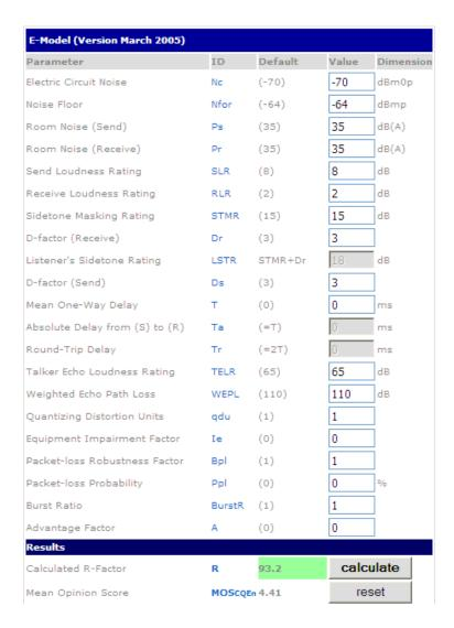
Figure 19 An E-model calculation tool
