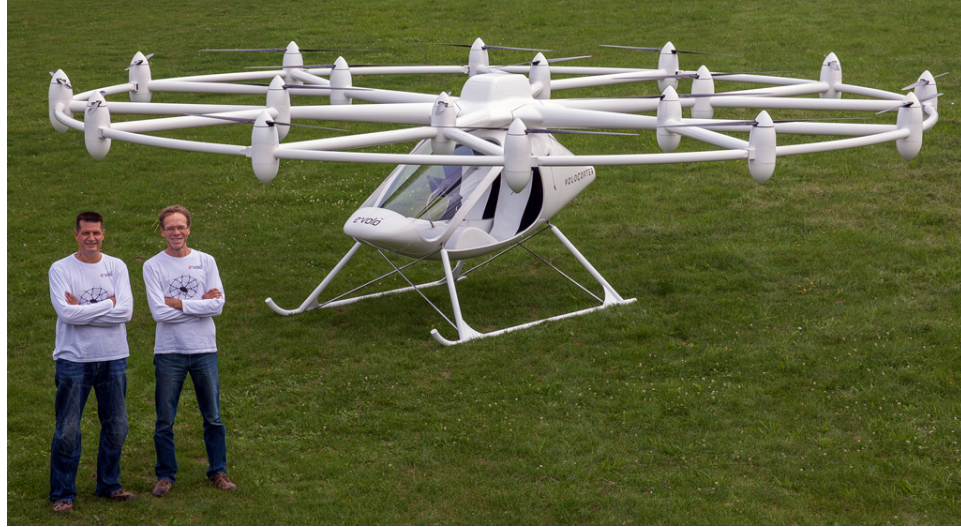
Figure 5: E-Volo all-electric helicopter concept. Eighteen motors and propellers are used to generate the required lift to transport two people at 50 kts [53].
