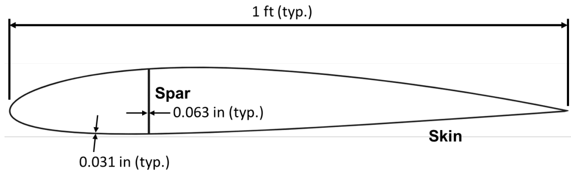
Figure 3.8: Scale representation of a typical wing cross section
