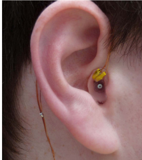
Figure 3.1: HRIR measurement apparatus.
