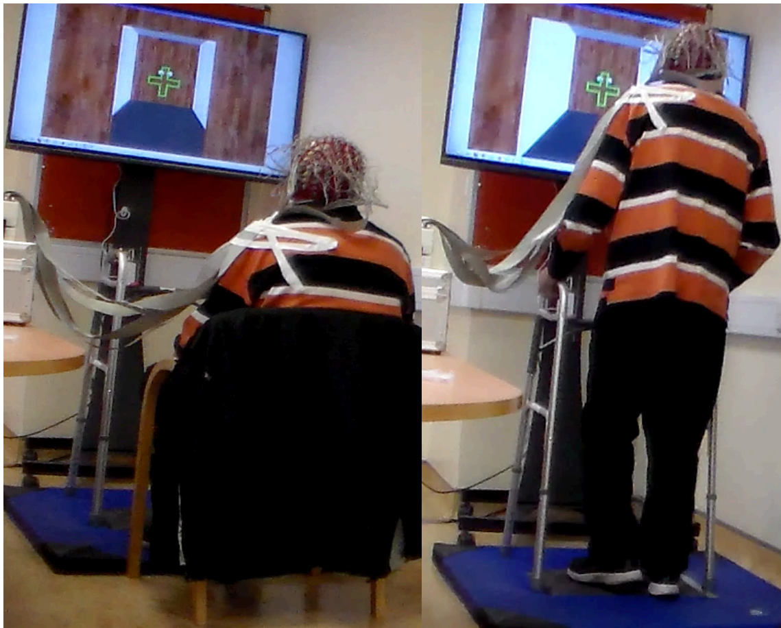
Figure 6.3. Two-stimulus oddball task sitting and stepping: Participant seated comfortably (left) and stepping in place (right) in front of LCD monitor with 128-channel EEG attached. Two-stimulus oddball task is presented superimposed on the virtual reality corridor.
