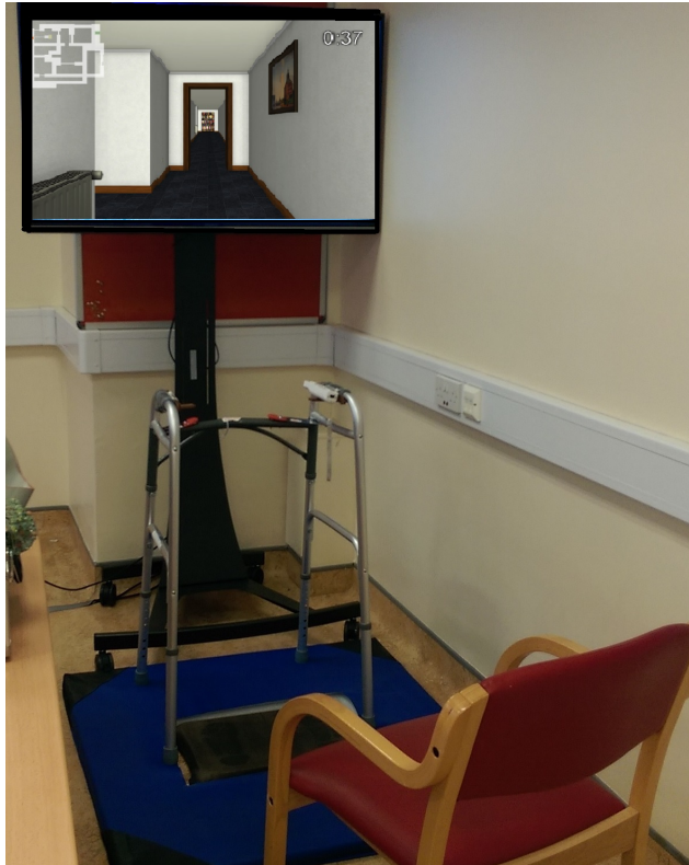
Figure 7.2. Experimental setup for Virtual Reality Maze: Virtual reality maze projected on 55-inch LCD screen with balance board (black) embedded in non-slip mat (blue). Walking frame provides safety support as well as housing remote controls.
