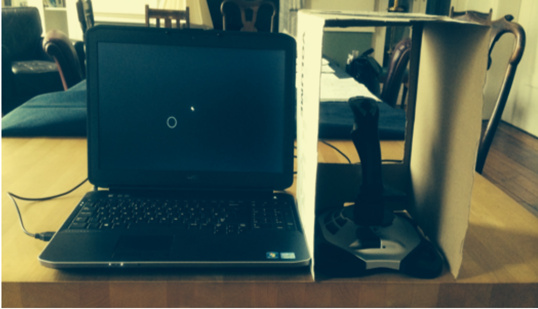
Figure 4.2 Experimental setup for motor skill acquisition task. The cursor and target are shown in this training exercise on a black background. Participants are asked to manipulate the joystick (hidden from view) in order to move the cursor into the target space in order to obtain the reinforcement signal. The cursor and/or target are shown or hidden, depending on the exact training exercise. During the Continuous Cue Experiment, the cursor is hidden and the target is shown. During the Movement Learning experiment, both cursor and target are hidden.
