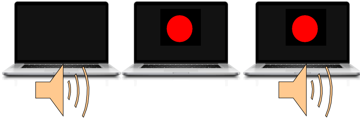
Figure 3.1. Unisensory and multisensory stimuli: Stimuli for auditory-alone (A, left), visual-alone (V, middle) and audiovisual (AV, right) conditions. The auditory condition consisted of a 1000-Hz tone (75 dB; rise/fall time 5 msec). The visual condition consisted of a red disc with a diameter of 3.2 cm (subtending 1.5 degrees in diameter at a viewing distance of 122 cm) on a black background. The audiovisual condition consisted of the auditory and visual conditions presented simultaneously. All stimuli were presented for 60 milliseconds.
